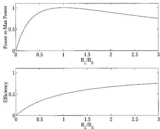
FIG. 2. (Top) power delivered to the load relative to maximum power  $v^2/4R_s$ , and (bottom) efficiency of power delivered to the load; both are plotted as a function of the load resistance to source resistance ratio  $R_L/R_s$ .
